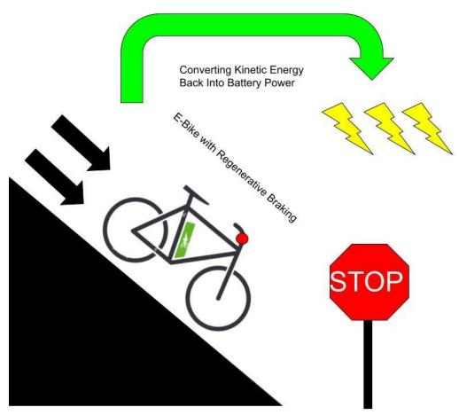
Fig 1: Example of Regenerative Braking Application
