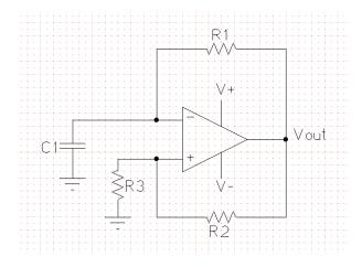
• Requirement 1: Produce a square wave at 1kHz with a +/- 100Hz margin of error.
