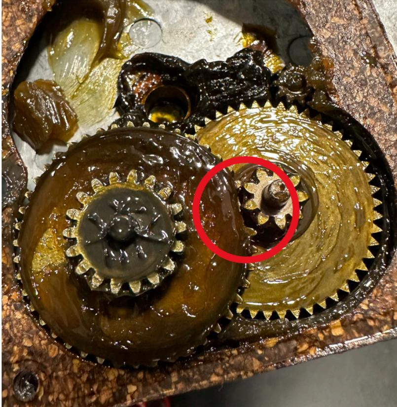
Figure 10: Broken gearbox
