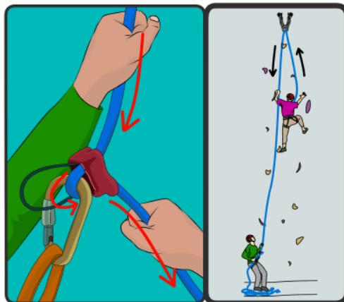
Figure 5: Typical top-rope climbing setup. In this example the belayer is using an ATC instead of a grigri, but the same principles apply.
