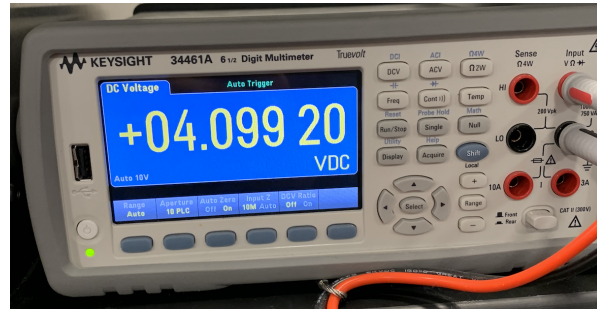
Figure 11: Battery Pack Voltage Reading
