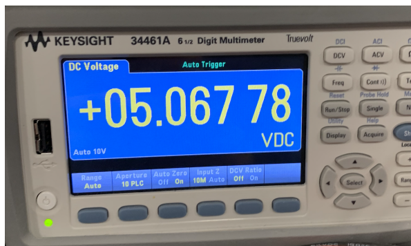
Figure 7: PCB 5V Output Reading
