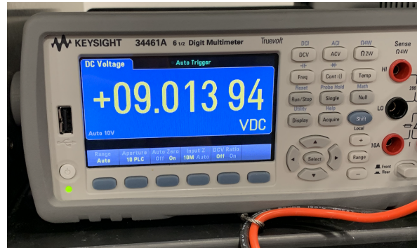
Figure 13: MP3429 Voltage Output Reading
