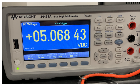
Figure 14: L78S05 and USB Receptacle Vbus Voltage Output Reading
