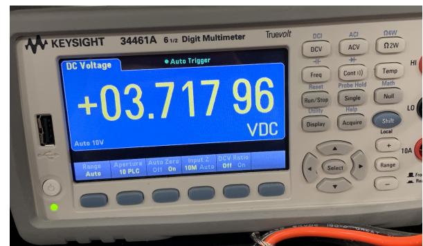
Figure 8: PCB 3.3V Output Reading
