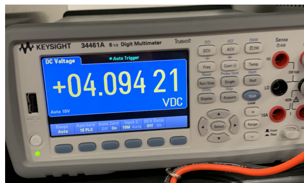
Figure 12: MP3429 Input Voltage Reading After the Power Switch is Closed
