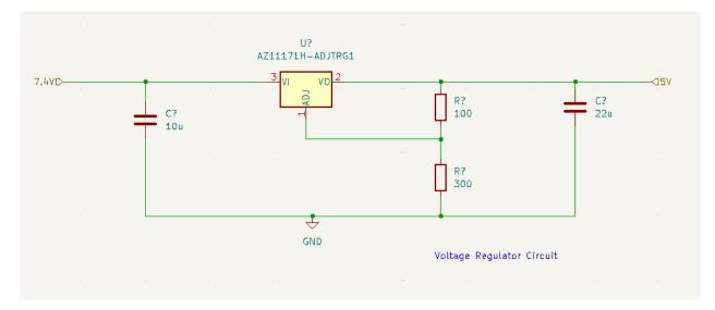
Figure 4: LDO circuit schematic.
