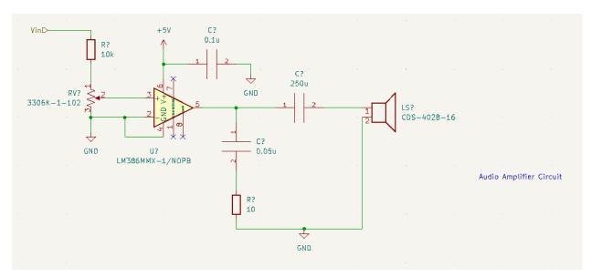
Figure 8: Audio amplifier circuit schematic.
