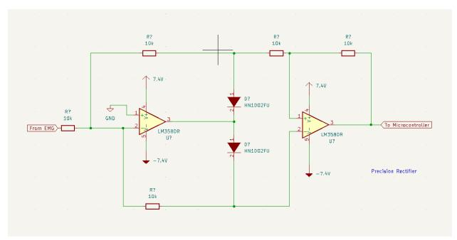
Figure 6: Precision Full Wave Rectifier circuit schematic.
