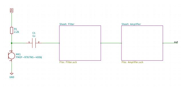
Figure 7: Audio detector circuit schematic.
