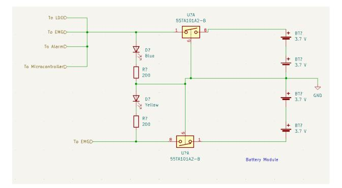
Figure 3: Battery Module schematic.
