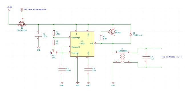
Figure 9: TENS Unit circuit schematic
