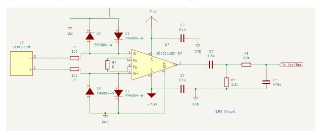
Figure 5: EMG circuit schematic.
