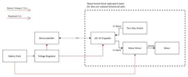
Figure 2: Block Diagram of Project Systems
