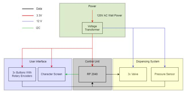
Figure 2: Block Diagram of Dispensing Machine
