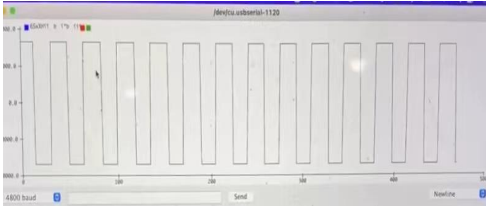
Figure 8. Test Results for Internal Test Signal (Square Wave from ADS1299)
