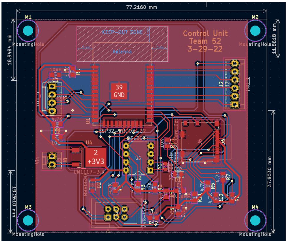
Figure 5. PCB of the control subsystem.
