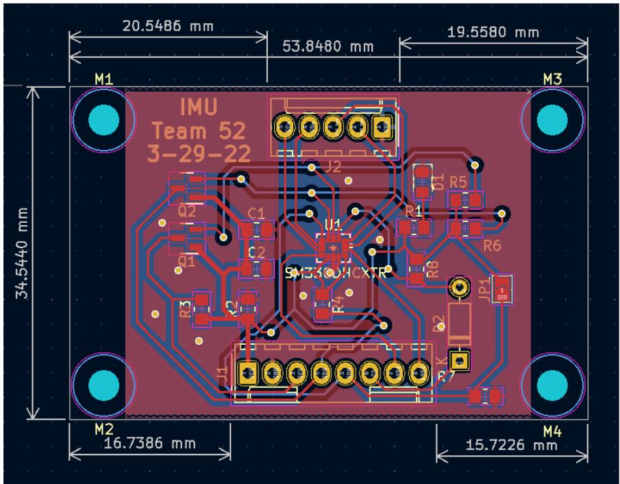
Figure 6. PCB of the IMU subsystem.
