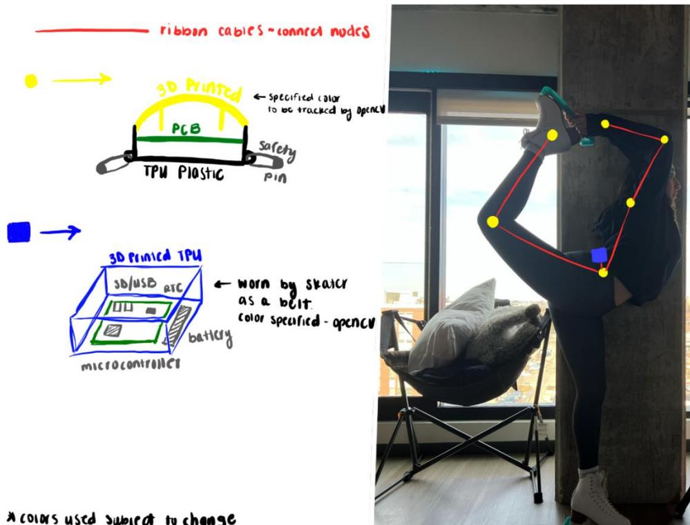
Figure 7. Visual aid with a more detailed breakdown of the wearable electronics system.
