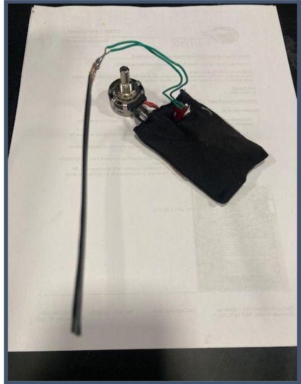
Fabricated PCB for Verification and Housed PCB
