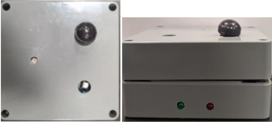
Figure 2 - CO 2 Sensor and PIR Sensor
