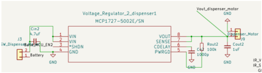
Figure 10. Voltage Regulator Circuit Schematic
