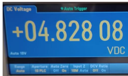
Figure 12 Typical output voltage of 5V Boost Converter
