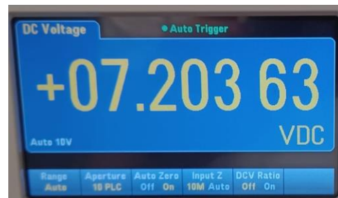
Figure 13 Typical output voltage of 7V Boost Converter
