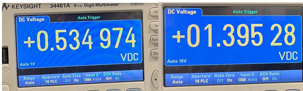
Figure 15 Analog Output without filtering and filtering respectively
