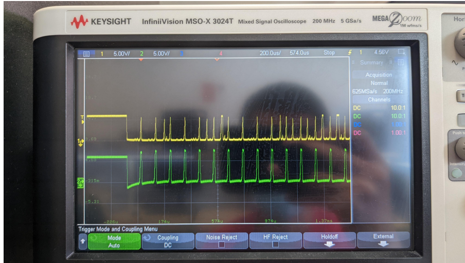
Figure 16: SCL (green) and SDA (yellow) from output of optoisolator
