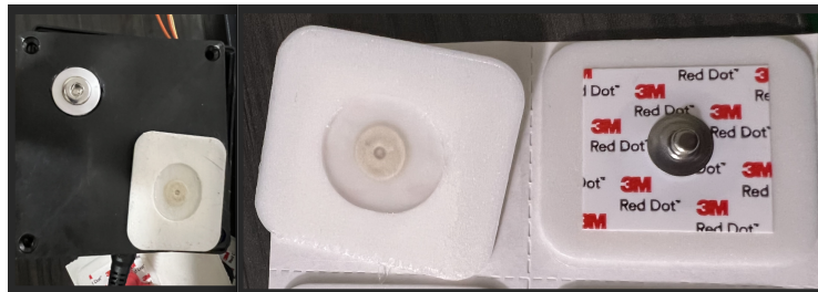
Figure 4. 3M 2650 multi-purpose monitoring ECG patches (right) and patches on the bottom of the device (left)
