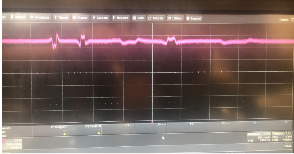
Figure 8: Negative and positive spike created when simulated bee enters and exits tunnel. Vertical scale of 500 mV/div and time scale of 500ms/div. First pair shows fast bee movement speed, second pair shows medium speed, and third pair shows slow speed.
