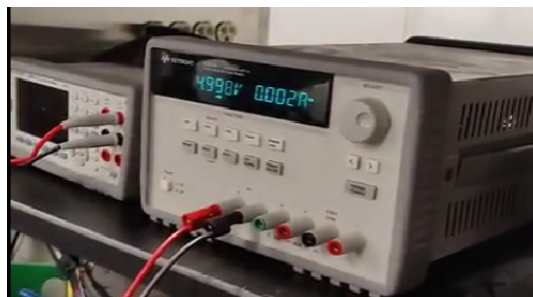
Figure 3.7: Sprayer pump current when not activated
