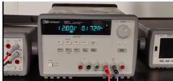
Figure 3.6: Current Drawn by Wiper Motor
