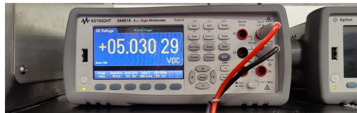
Figure 3.4: Output of microcontroller supply regulator when mounted on PCB.
