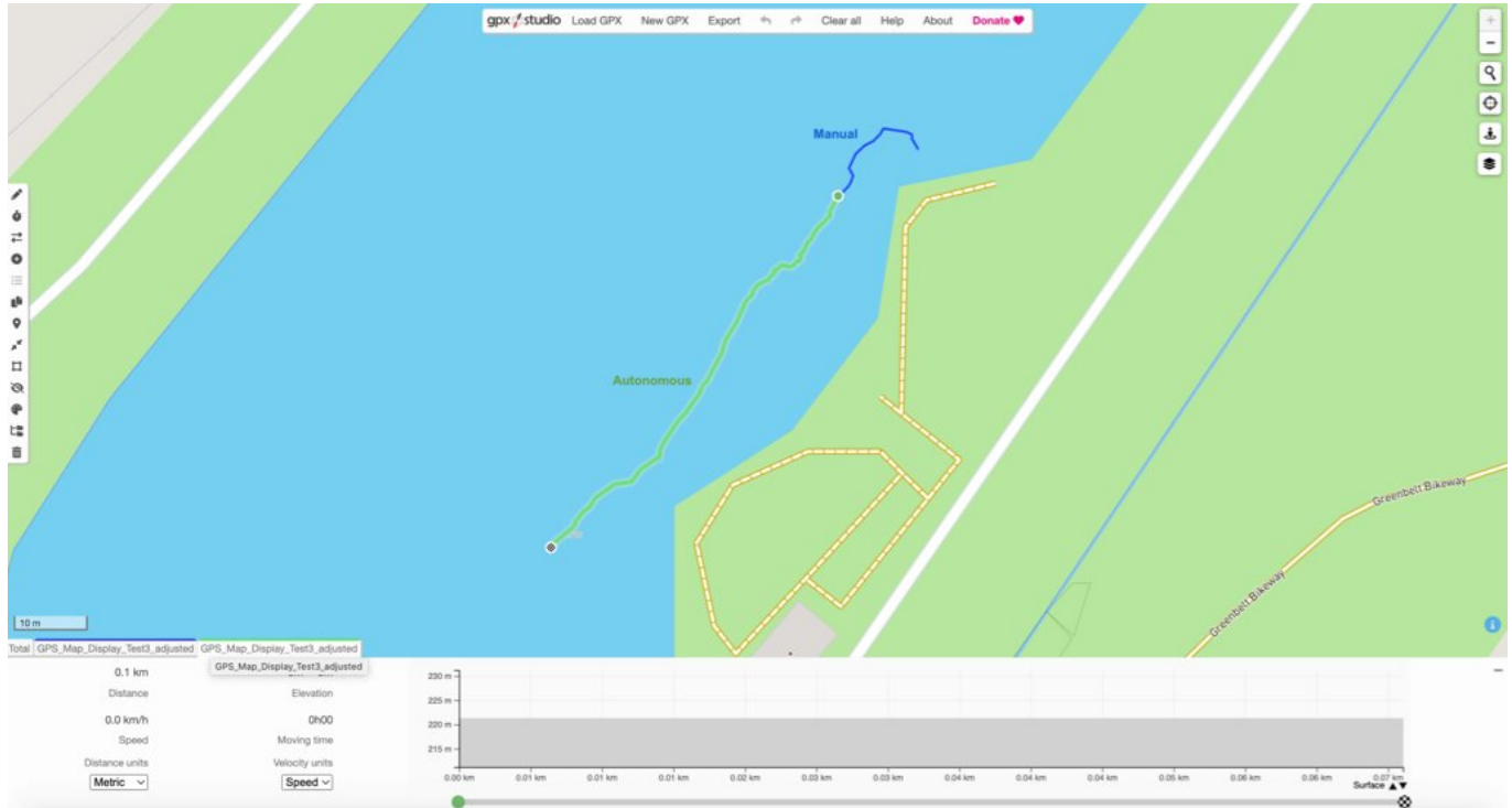
Figure 11: Sailboat movement (green: autonomous mode, blue: manual mode)
