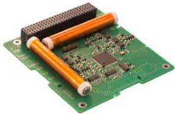
Example of a 2-axis COTS magnetorquer-based ADCS module.
