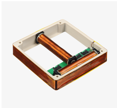
Example of a 3-axis COTS coil system.
