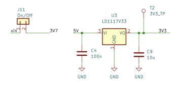
Figure 2.3.1.1 Linear Voltage Regulator
