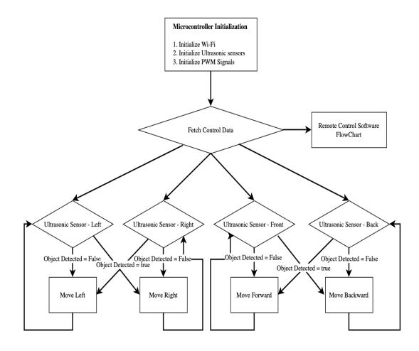
The auto mode of the Fun-E-Mouse is using the four ultrasonic sensors to detect any nearby object within 10cm distance. Let False denote no objects detected in front of the ultrasonic within 10cm. Let {Right, Left, Forward, Backward, Stop} denote the direction of the Fun-E-Mouse, and Let Choose{} denote a random function that picks any given direction. The following table describes how the Fun-E-Mouse operates in the Auto Mode.
