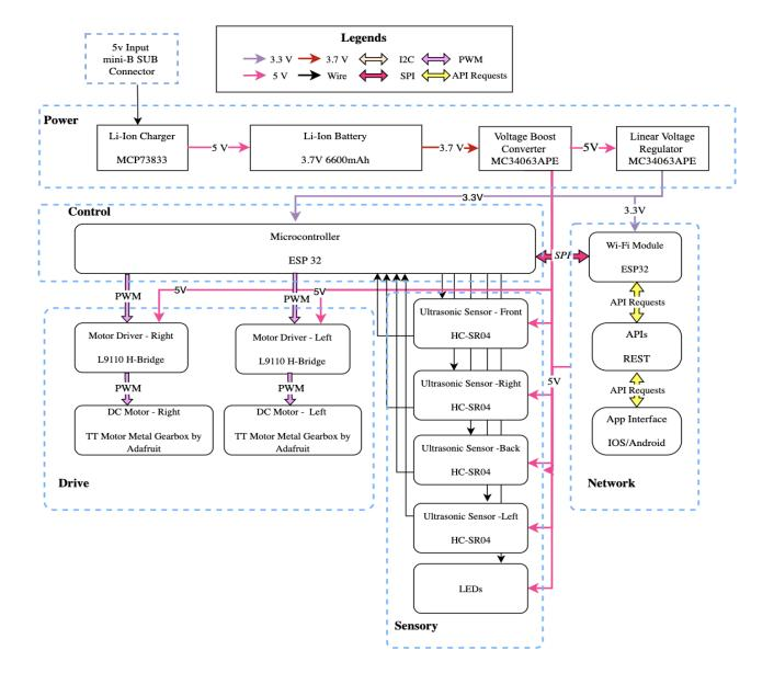
Figure 2.1 Block Diagram of the Fun-E-Mouse
