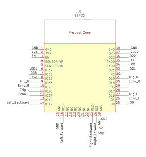
Figure 2.3.2.1 Esp32 Schematic
