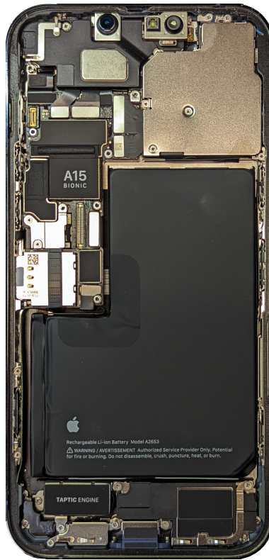
Figure 1: A teardown view of the iPhone 13 Pro Max.
