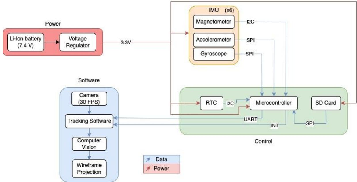
Figure 2. Block diagram breaking down the subsystems of the project.
