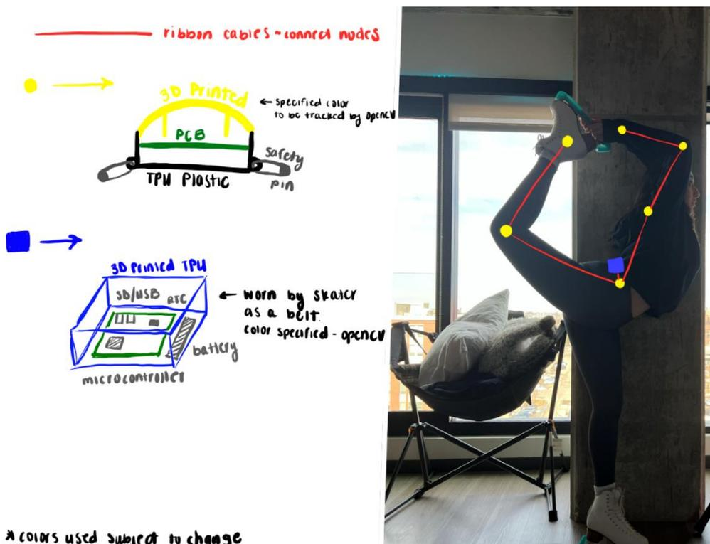
Figure 5. Visual aid with a more detailed breakdown of the wearable electronics system.
