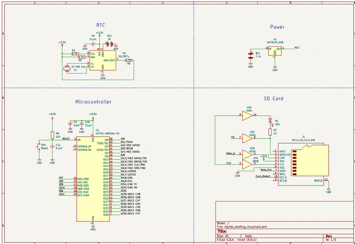
Figure 3. Schematic of the control subsystem.
