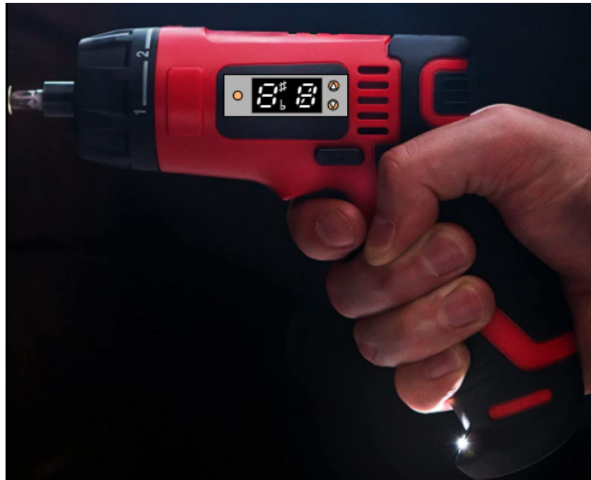
Figure 3: A mock-up using a electric driver [3] that would give the correct amount of torque ( \sim 10Nm ).
