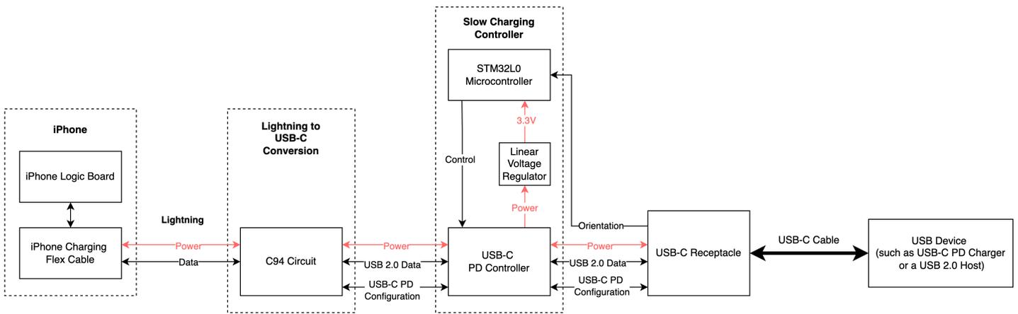
Note: the connections labelled as "Power" without a voltage specification may carry anywhere between 5V and 12V, depending on the negotiated **VBus** voltage as per the USB-C Power Delivery specification.
