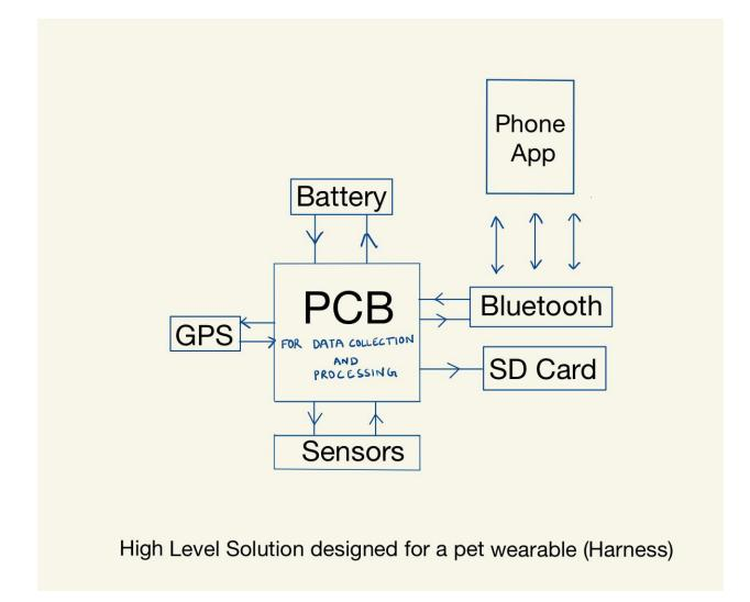
data collected by the accelerometer will be used to find the displacement in order to find the location of the pet. After collecting and calculating all the relevant data, meaningful results will be generated for the users which they can access using phone applications.
