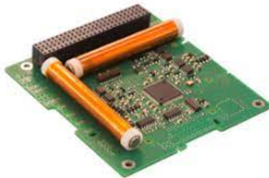
Figure 1: A photograph of a commercial off-the-shelf (COTS) 2-axis ADCS module for cubesats. Roughly 10cm on a side, this is comparable to what we are building. Unlike this unit however, our module is compliant with LASSI hardware, making it far more useful to UIUC interdisciplinary endeavours.
