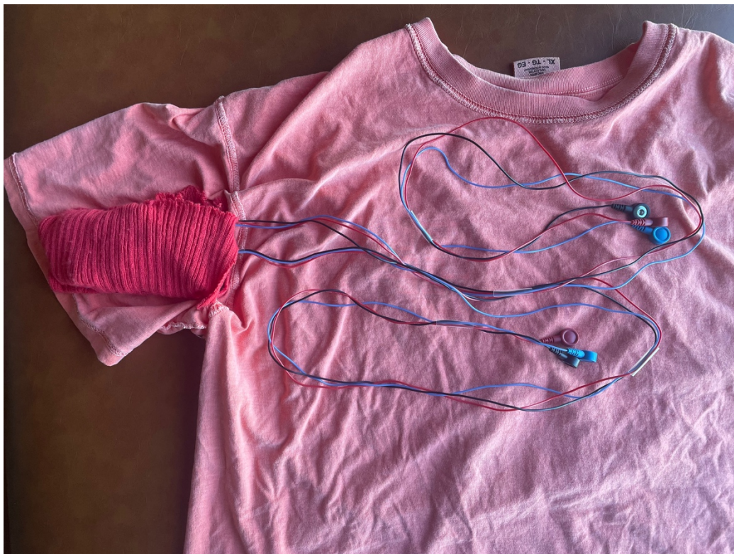
Figure 17. T-shirt with sewn on PCB on the sleeve and the outlets for the electrode wires; inside view
