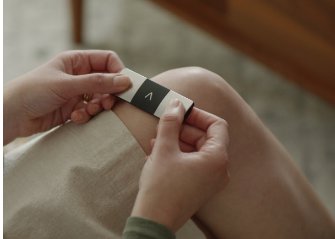
Figure 4. KardiaMobile, single-lead wireless solution [10]
