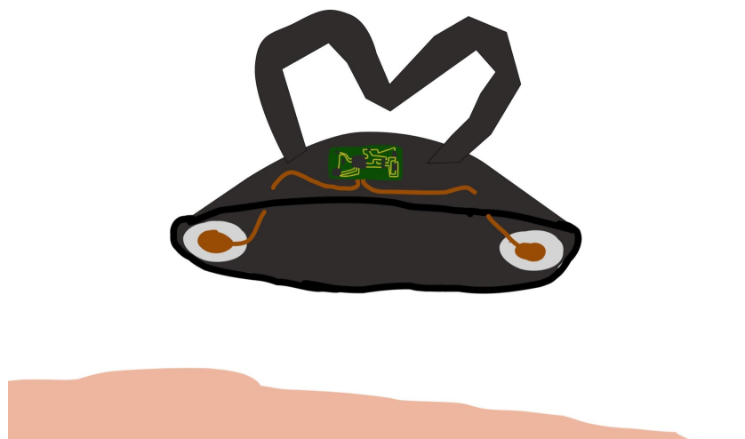
Figure 8. Physical design of suction cup system with handle and visible attached PCB above the skin
