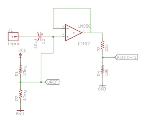
Output Buffer circuit schematic:
