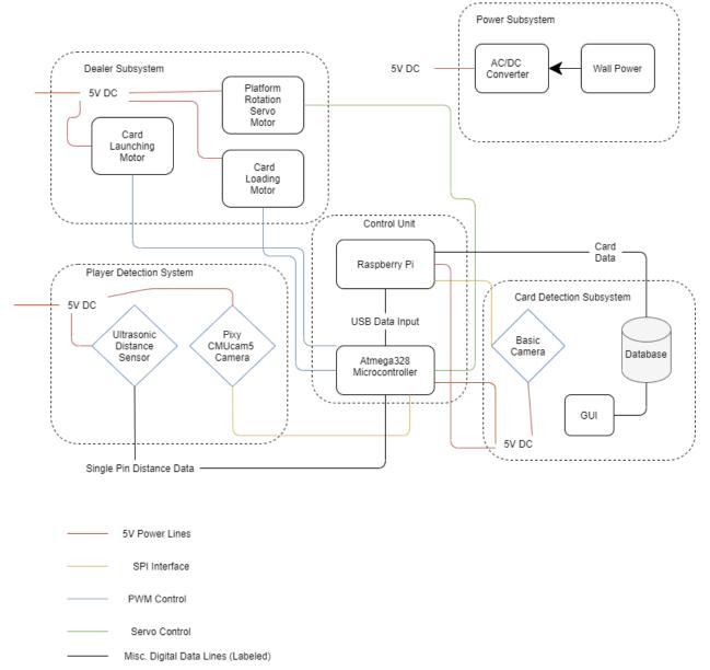
The block diagram outlines 4 different portions that will work together in order to fulfill the high level requirements. The power subsystem consists of an AC/DC converter that can supply 5V DC power to all our components. The dealer subsystem is the section that removes a single
