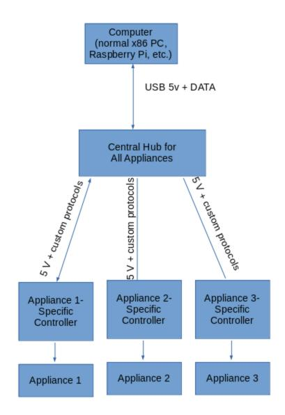
Appliances may either be powered by the hub, which can either be powered by the computer or by an external power supply. Each of the appliances can also have their own power supply, depending on the power requirements of the appliance.
