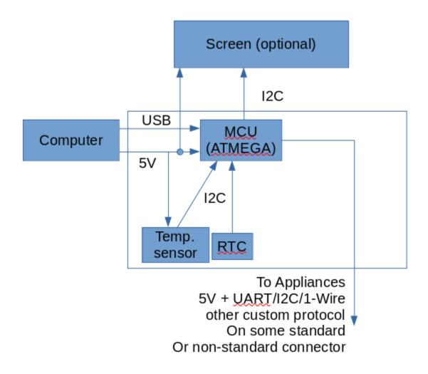
This subsystem is used to interface the simple protocols used by the appliances with the USB on the computer. There are a few other chips, mostly to provide auxiliary logic to the microcontroller where it is required (e.g. temperature sensor for a thermostat appliance, and an RTC to support schedules (e.g. to turn on and off an appliance at a certain point in time))
