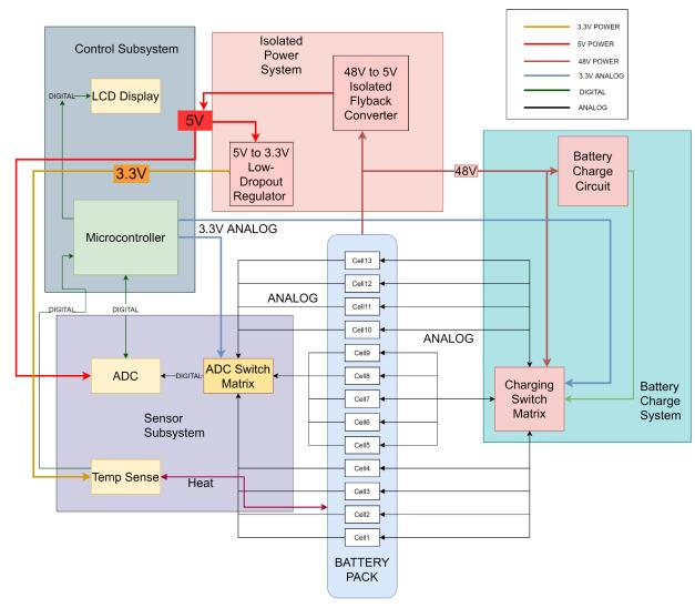
The project consists of a Control Subsystem, Sensor Subsystem, Isolated Power System, Battery Charge System and the battery itself.
