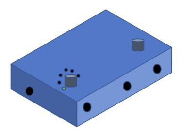
We envision the chassis being of dimensions equal to or less than (20 cm, 15cm, 8cm), and having 2 female ½ inch connectors, one MIDI out, and one 9V DC power input. We want the dimensions to be such that it fits on a standard guitar pedal board and is compatible with the rest of the guitarist's signal chain. In terms of controls, we want the guitarist to be able to specify the harmony they would like to generate as well as the type of waveform (from square, sawtooth, or sinusoidal).
