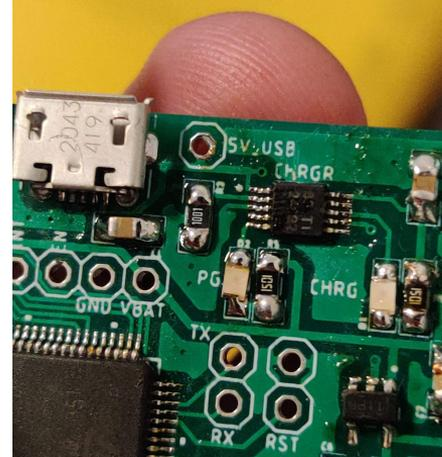
Close-up of charger & MCU soldering
