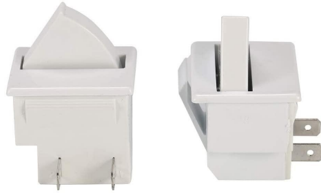
Figure 3. Door switch. This switch is ON when the switch is not being pressed, and OFF when pressed.
