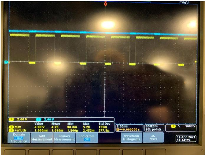
Pictured Left: Oscilloscope Reading of 1990us Pulse Width
