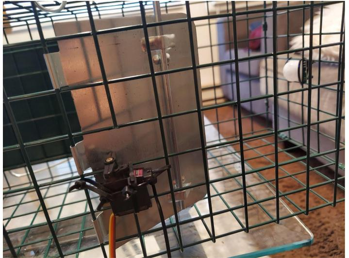
*Pictured Right: Servo Restricting the Trap's Pressure Plate*
