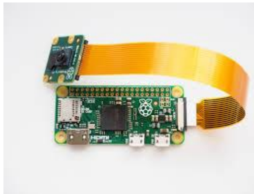
Figure 4: Raspberry Pi zero connected to the camera module
