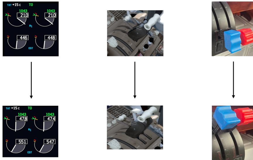
Figure 1: Illustration of device operation. Multi-function display (MFD) of the aircraft (left). Real looking of the throttle quadrant (middle). Flight simulator throttle quadrant (right). The MFD, real throttle quadrant, and simulator throttle quadrant on the same row represent the same the engine thrust setting.
