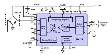
Figure 4. Typical weight scale application block diagram [8]
