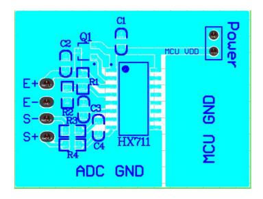
Figure 7. PCB board layout for HX711 [8]
