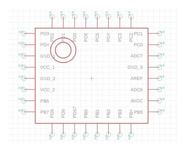
Figure 8. Eagle ATMega 328P\_AU Schematic
