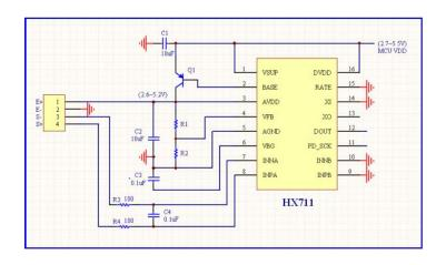
Figure. 6 PCB board schematic for HX711 [8]
