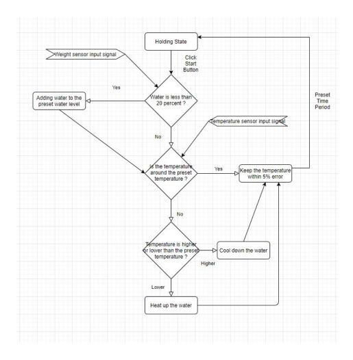
Figure.9 Software control flowchart
