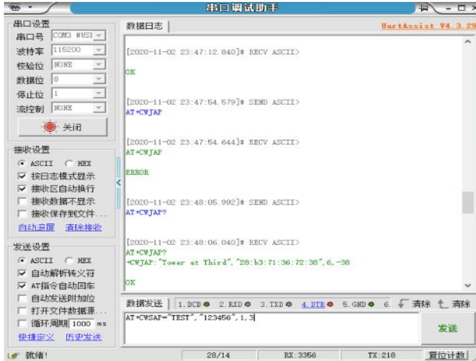
Figure 11: Test for ESP8266 to Connect to Local WiFi
