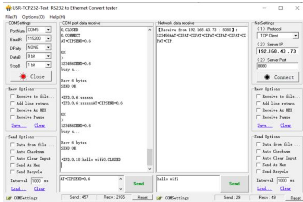
Figure 12: Test Bi-direction Communication of ESP8266
