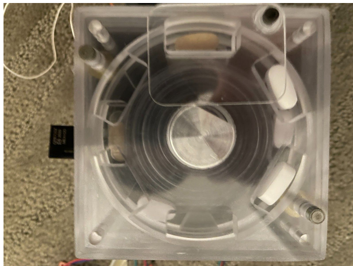
Figure 4: Final Location of PE Sensor ( the black box on the left)
