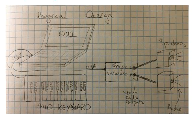
The Physical design will be small and minimal, as the only fixtures required on the box itself will be a USB port and stereo audio outputs. A black metal enclosure with just those items and perhaps an insignia is all that will be necessary.
