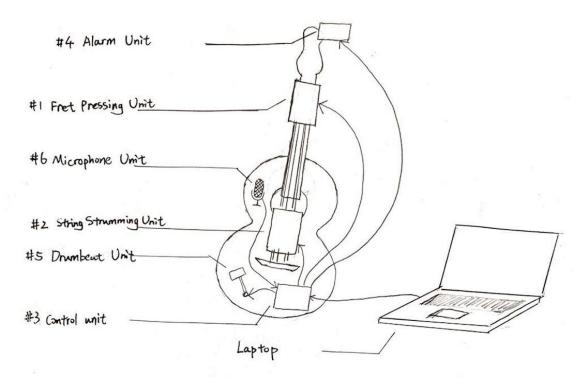
The six units of our design should be able to attach to any type of guitar as the above graph shows. The Control Unit will be programmed through the laptop, and is also in charge of sending records from the Microphone Unit to the laptop.
