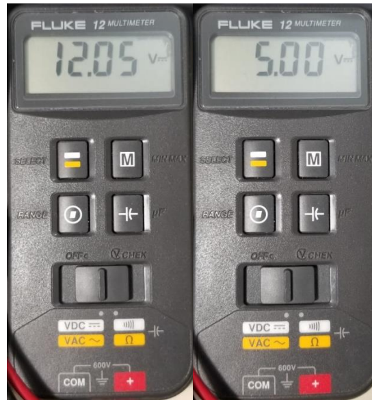
Figure 12: Multimeter Display of Input/Output Voltage from Voltage Regulator
