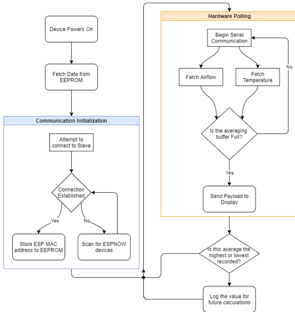
Figure 8. Sensor Controller algorithm, it is assumed that the device has been properly calibrated.
