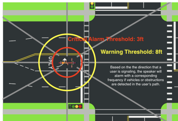
Figure 1: Diagram showing the regions that each ultrasonic sensor will cover as well as the conditions under which varying alarm tones will be made.
