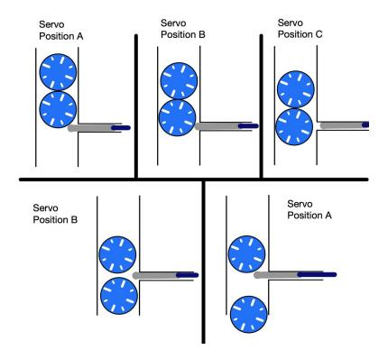
Figure 11. The lever positions based on the servo motor positions.
