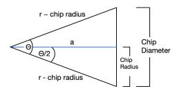
Figure 9. Isosceles triangle formed by the chip's radius,  $\Theta$ , and the chip's diameter.
