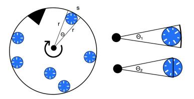
Figure 8. Diagram showing angle  $\Theta$  that covers a poker chip. Rotating disk has radius r, and s is the arclength of that angle  $\Theta$ . Diagram also shows simplification going from solving  $\Theta_1$  to  $\Theta_2$ .
