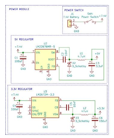
Figure 3. Power supply circuit schematic.
