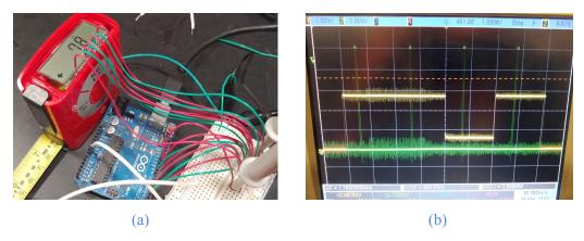
Figure 15. Tape measure (a) testing setup and (b) oscilloscope readings from display.
