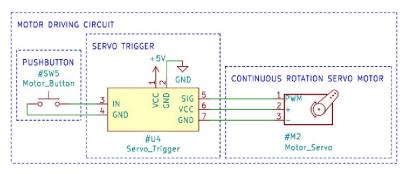
Figure 5. Motor driving circuit schematic.
