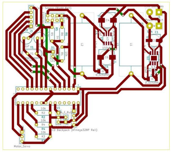
Figure 7. Console PCB layout.
