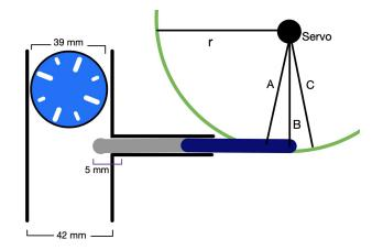
Figure 10. Diagram of chip size compared to the tube as well as the servo disk connected to a lever to control chip traffic in the tube.
