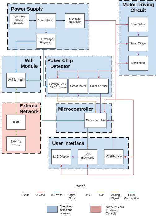
Figure 2. Block diagram.
