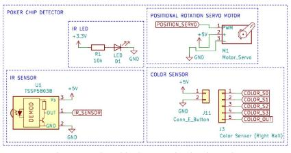
Figure 4. Poker chip detector circuit schematic.
