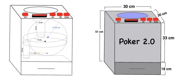
Figure 1. Inside view of console (left) and outside view of console (right).
