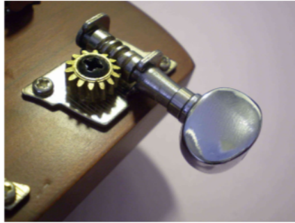
Figure 2.7.2 Tuning Knob Mechanism [13]
