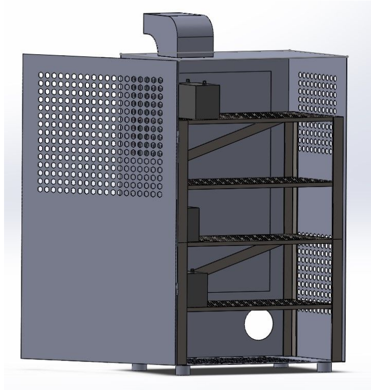
Figure 5: Draft of the battery bank storage case
