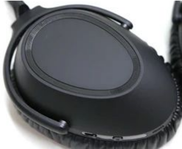
Figure 4. Example of the planned button layout and closed back design for our drivers
