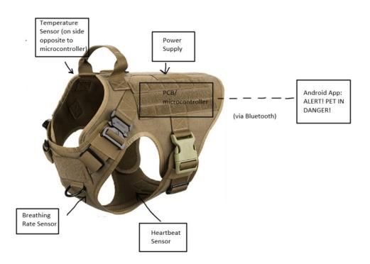
The physical design above is a high level overview of our *Pet Guardian* design. It includes the sensors, power supply, and microcontroller, as well as the software interface. For budgeting purposes, we can make use of already owned Rabbitgoo size large dog harnesses if needed. However, we are planning to use a tactical dog harness in order to have enough area to fit the sensors, power supply, and microcontroller of our choosing.
