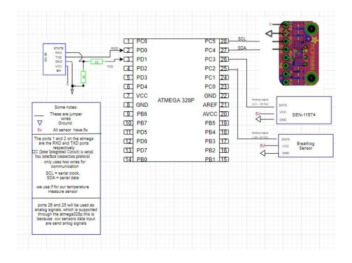
Connection of Sensors and Microprocessor
